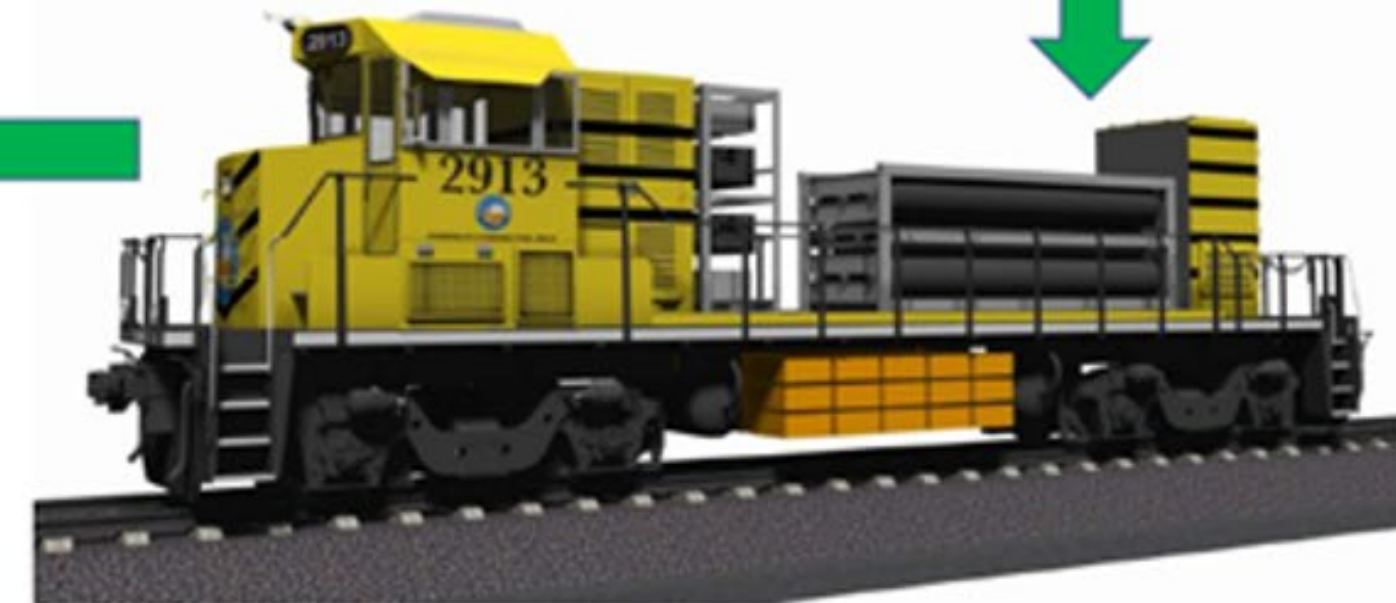
Repowered with 200 kW Fuels Cells, 222 kg Hydrogen Storage, and 500 kW-hr Battery Storage Installed
